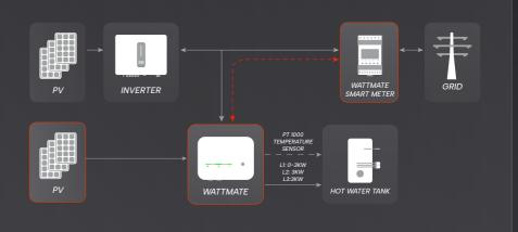
\*Direct PV input and grid input cannot work at the same time.
