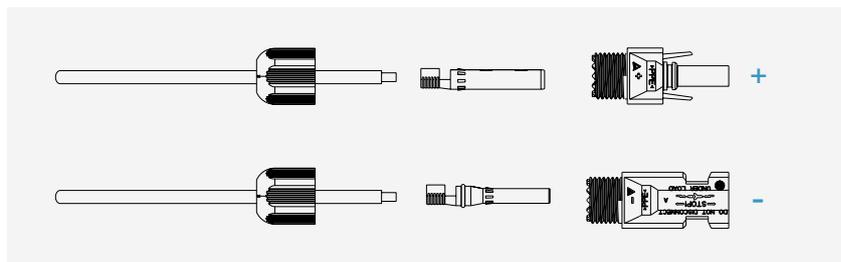
4) Insert the DC cable through the DC connector nut into the metal terminal and press the terminal with a professional crimping plier (pull back the cable with some power to check if it's tight enough).
