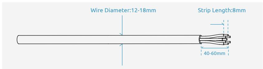
2) Insert the stripped AC cables through the AC connector cover in the sequence.
