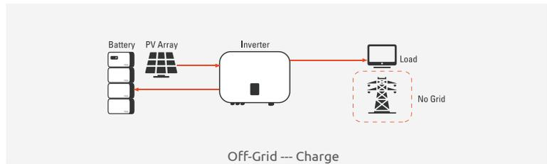
When the power from PV is weak, the battery will discharge to supply back-up loads together with or without PV.
