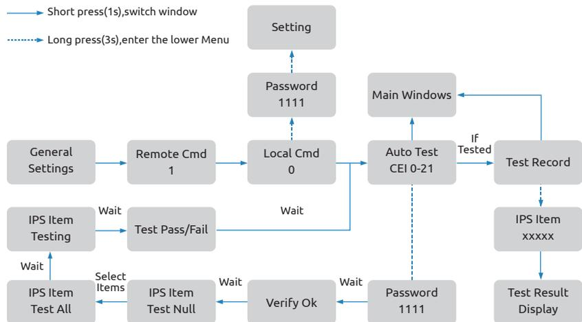
The auto test will start when the correct test item is selected, and the test result will be displayed on the screen when it finished. If the test success, it will display "Test Pass", otherwise will display "Test Fail". After each item tested, the inverter will reconnect to the grid and automatically start the next test item according to the requirements of CEI 0-21.
