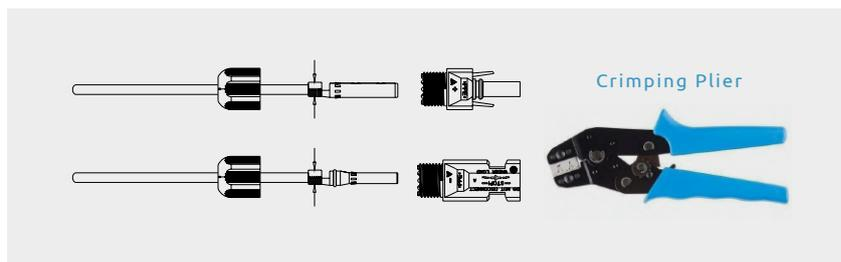
5) Insert the positive and negative cables into the corresponding positive and negative connectors, pull back the cable to ensure that the terminal is tightly attached in the connector.
