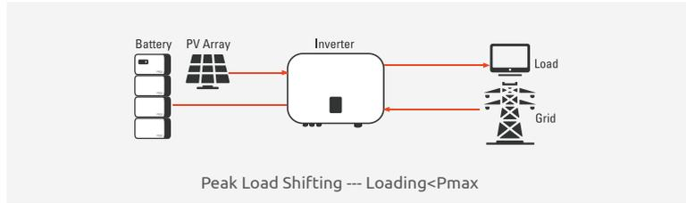
In this working mode, set the Pmax from grid in the App can realize the “Peak Load Shifting”. When the loads consumption less than the Pmax, loads are supplied by the PV array and grid together.
