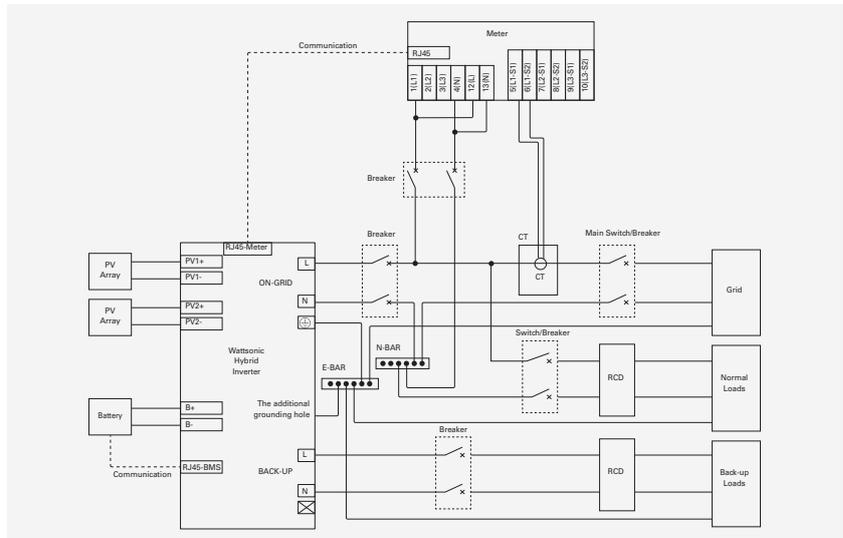
This diagram is an example for Australia and New Zealand. Neutral line of AC supply must not be isolated or switched.
