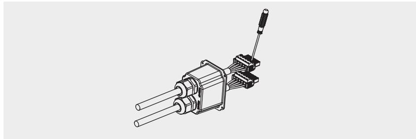
5) Insert the assembled AC connector to the corresponding AC port in the inverter.
