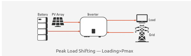
\* To realize the “Peak Load Shifting” function, the load power that exceeded Pmax has to be within the inverter max output power, otherwise, the inverter will only output the max power which allowed.
