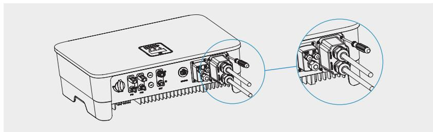
7) Screw up the rubber ring and anti-water cap to make sure the AC connector is well sealed.
