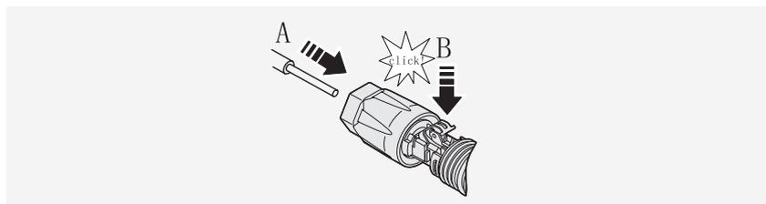
5) Push the battery connector to the thread joint, and use an open wrench to lock the connector in a torsion of 2Nm tightly.
