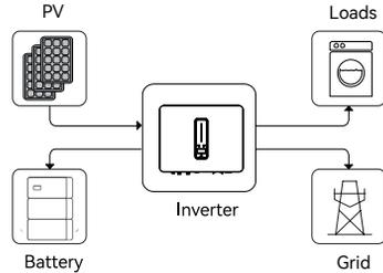
When the PV power is insufficient, the battery will discharge to supply loads, and the grid will join in if the battery is not enough to supply loads.
