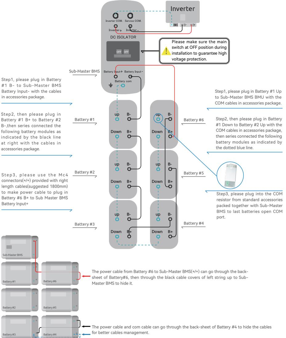
Step1, please plug in Battery #1 B- to Sub-Master BMS Battery Input- with the cables in accessories package.
