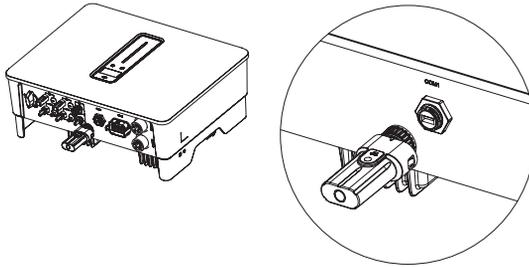
Figure 5-10 Monitoring device installation
