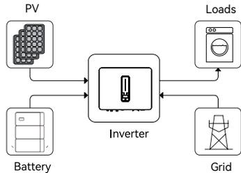
**Peak load Shifting (Load Shifting)**
