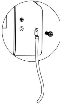
Figure 4-8 Grounding terminal connection
