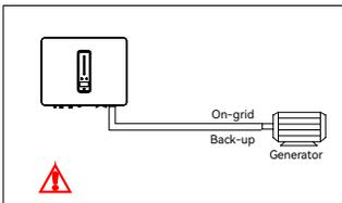
The on-grid and back-up side cannot be connected to and generator directly. For advanced applications, please contact our after-sales department.
