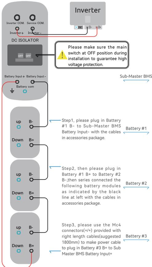
Battery communication cables connection
