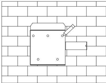
Figure 4-5 Marking hole position using installation bracket
