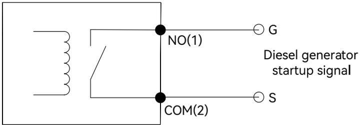
Figure 5-26 Generator Control connection diagram
