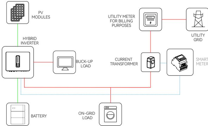
Figure 3-1 Schematic diagram of hybrid system
