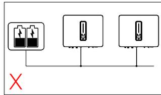
One battery bank cannot be connected to multiple inverters.
