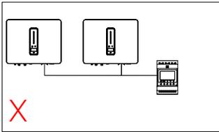
One meter cannot be connected to multiple inverters. Different CTs cannot connect to the same line cable.
