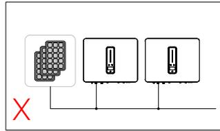
Single PV string cannot connect to multiple inverters.
