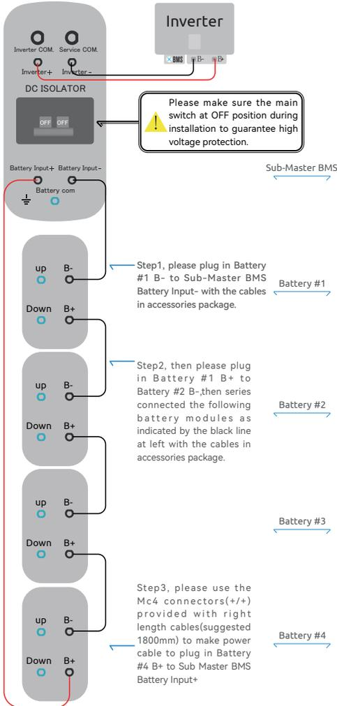
Battery communication cables connection
