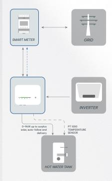
Measuring available surplus solar by means of WattMate smart meter installed at grid side, the WattMate minimizes the power demand of the electric element in the water heater / hot water storage tank, consequently avoiding the need to draw electricity from the grid, plug and play.
