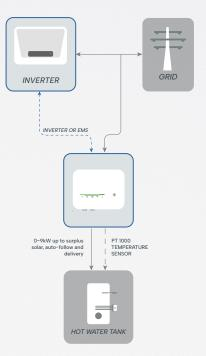
Set up direct communication to inverter via Modbus protocol, Wattmate can always follow real-time PV generation and deliver surplus solar to water heating automatically.
