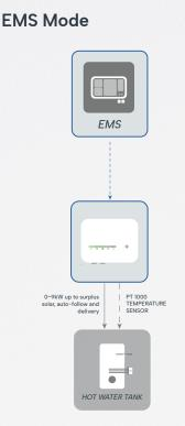
Thanks to standard Modbus RTU/TCP-IP protocols integrated, Wattmate can be seamlessly integrated by any external control devices.
